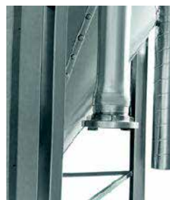
Feed truck connection
